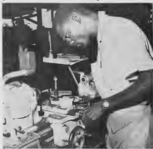
THE DELICATE job of turning down a shaft on the 10-inch engine lathe to tolerances of .0005 of an inch is performed by E. Beyde, tradesman B. E TRABAHO dedicado di pasa un shaft ariba e engine lathe di 10 inch te tolerancia di .0005 di un inch ta worde haci door di E. Beyde, tradesman B.
